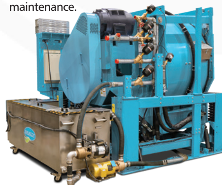
650 N2 Open Pocket Washer/Extractor with the washing capacity of 650 lbs with a width of just 106 inches.
